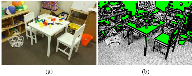
FIGURE 6. (a) An input image and (b) its gradient map, where green pixels represent the non-textured region \mathcal{P}_{NT} .
