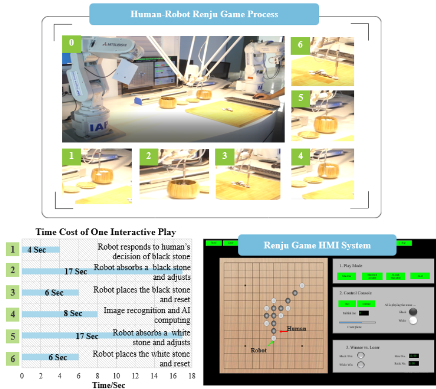
FIGURE 11. The process of Man-machine gobang game, the time cost and the monitoring interface.
