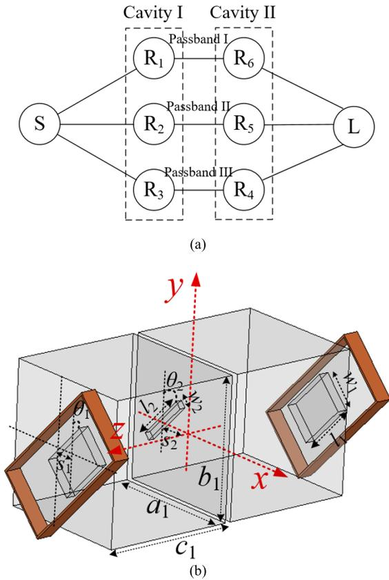
FIGURE 8. Schematic of the 2nd-order triplet with in-band-TZs. (a) Topology, (b) geometrical structure.
