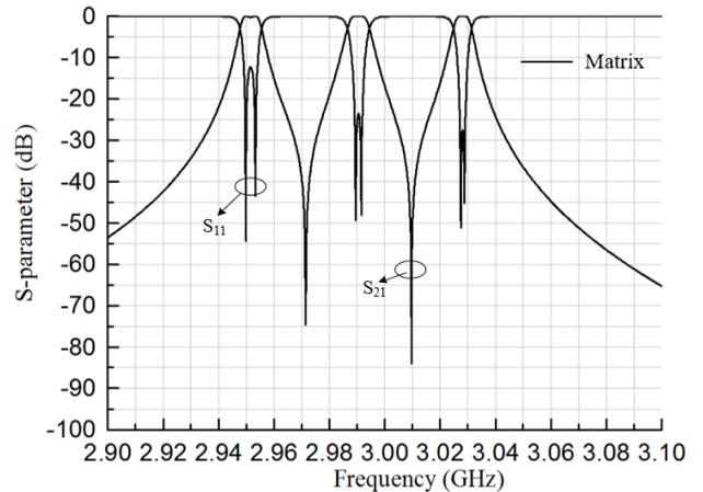
FIGURE 9. Calculated S-parameter frequency responses from the triple-band coupling matrix (10).
