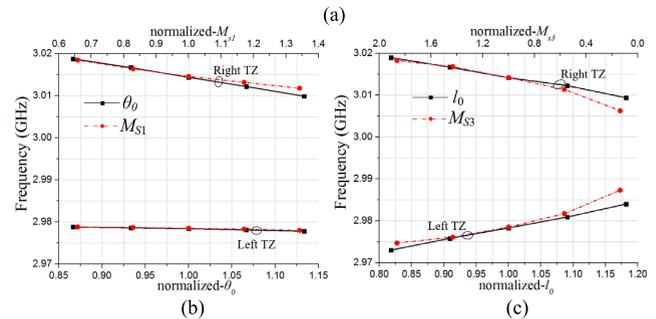
**FIGURE 7.** (a) Calculated S-parameter of the triplet with in-band TZs. (b) Variation in frequency of two TZs with respect to  $M_{S1}$  and  $\theta_0$ . (c) Variation in frequency of two TZs with respect to  $M_{S3}$  and  $l_0$ .
