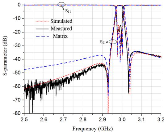
**FIGURE 6.** Comparison among the M-matrix calculated, measured, and simulated frequency responses of the proposed triple-mode cavity filter in Fig. 5.
