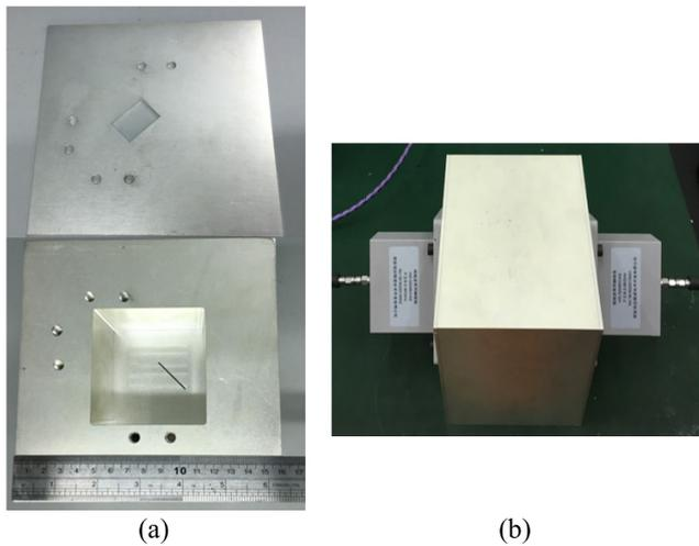
**FIGURE 10.** Photographs of the fabricated dual-cavity triple-band cavity filter. (a) Internal view, (b) external view.
