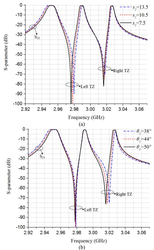
**FIGURE 12.** (a) Variation in location of TZs with respect to the  $s_2$  value. (b) Variation in location of TZs with respect to the  $\theta_2$  value.
