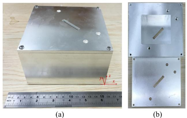
FIGURE 5. Photograph of the fabricated triple-mode cavity bandpass filter. (a) External view, (b) internal view.
