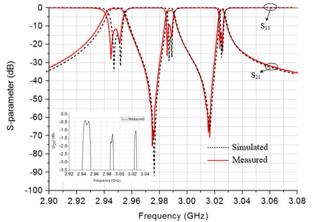
**FIGURE 11.** Comparison between the simulated and measured frequency responses of the dual-cavity 2<sup>nd</sup>-order triple-band filter.
