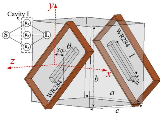
FIGURE 3. Geometrical structure of the designed triple-mode bandpass filter.
