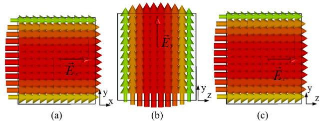
FIGURE 4. Electric field distributions of three modes. (a) TE<sub>011</sub>, (b) TE<sub>101</sub>, (c) TM<sub>110</sub>.
