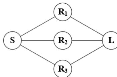
**FIGURE 1.** Basic coupling topology of a triplet for design of the proposed filter.
