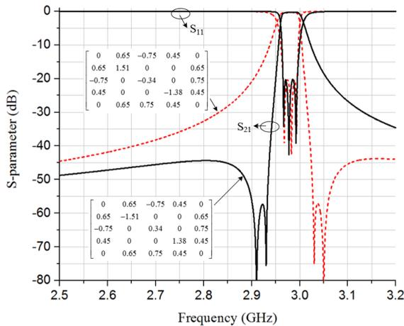
FIGURE 2. Calculated S-parameters of the proposed filter in the 1<sup>st</sup> and 2<sup>nd</sup> cases.
