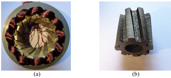
FIGURE 5. Skewed motor structure [36]. (a) Skewed stator. (b) Skewed rotor.
