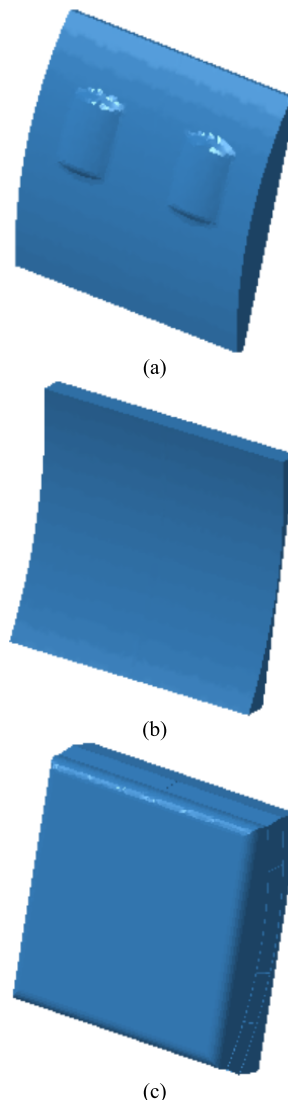
FIGURE 2. Computational model of the transmission loss of skin panels. a) Anechoic chamber. b) Reverberation chamber. c) AML model.
