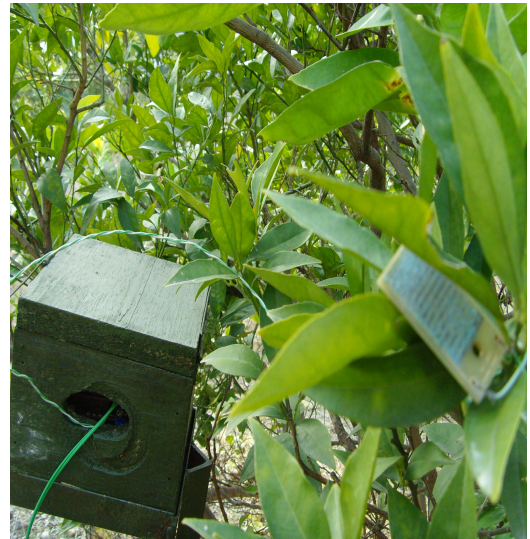
FIGURE 4. Leaf wetness sensor deployment near plant leaves.
