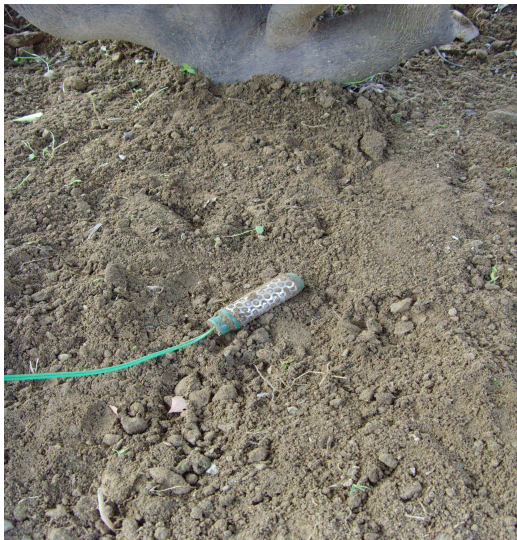
FIGURE 3. Deployment soil moisture sensor in real agricultural environment.
