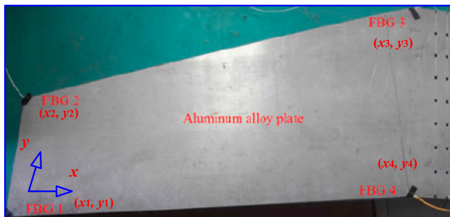
FIGURE 2. Aluminum alloy plate with FBG sensors stuck on [36].
