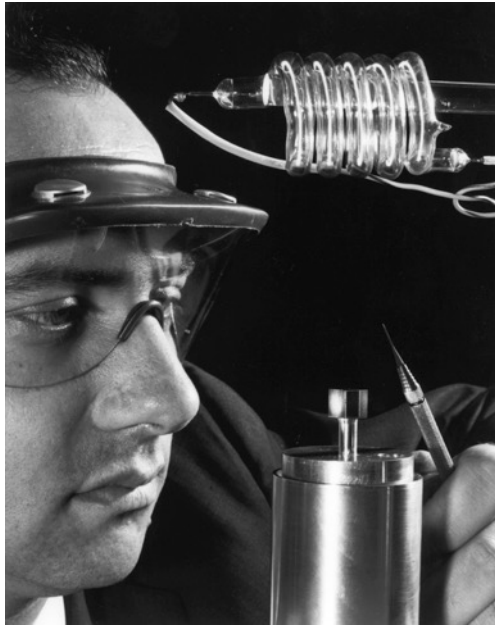
FIGURE 17. Theodore H. Maiman with the main components of the ruby laser. He preceded more credited physicists by developing the device at Hughes Aircraft Company in 1960. (Photo courtesy of HRL Laboratories, USA).
