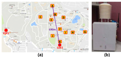
FIGURE 1. PM2.5 detection in NCTU campus. (a) The NCTU campus map with 11 PM2.5 sensors and 2 LoRa gateways. (b) An outdoor PM2.5 sensor device.
