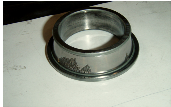
FIGURE 3. Bearing vibration inner race fault.
