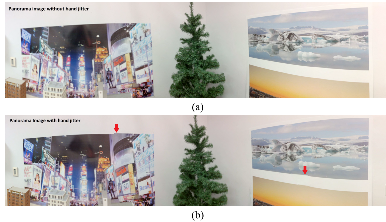
FIGURE 7. (a) The panoramic image captured without hand jitter. (b) The panoramic picture captured with hand jitter.
