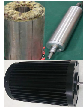
FIGURE 19. The prototype of the optimized motor.
