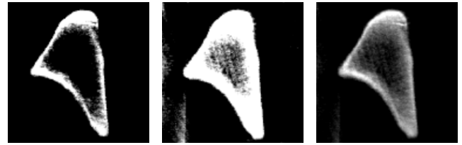
FIGURE 9. The influence of window level and width on the distribution of gray values in an image: 1150/190 (left, used in our system), 890/190 (middle); 1150/760 (right).
