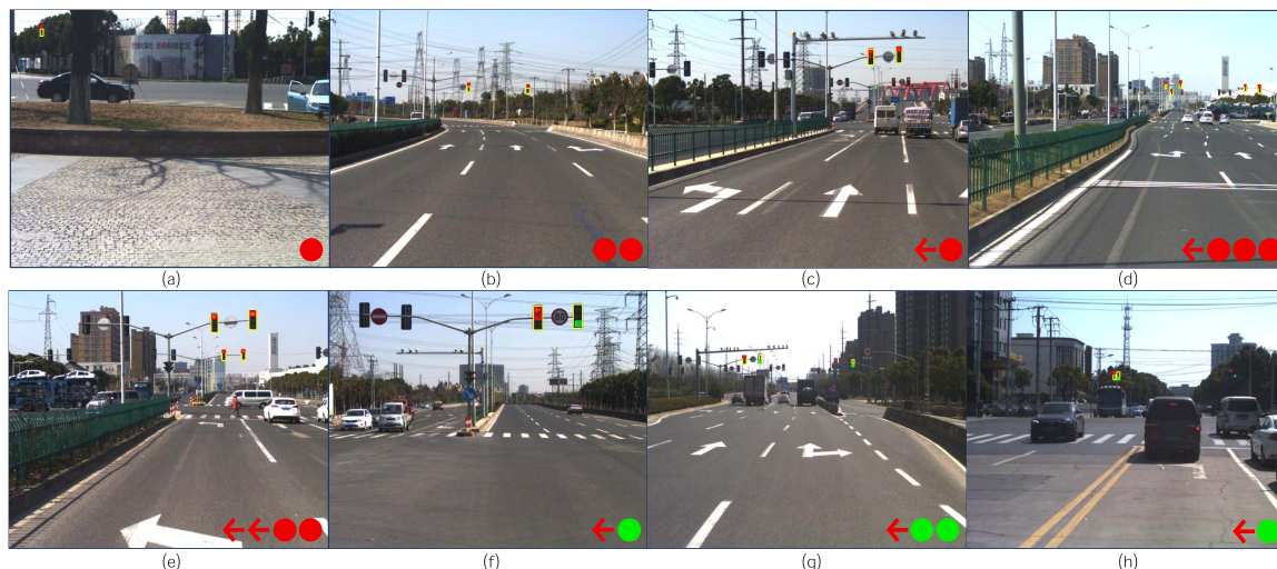
FIGURE 15. Traffic light detection results. (a-b) Traffic lights with complex background. (c-h) Detection results under different traffic scenes.
