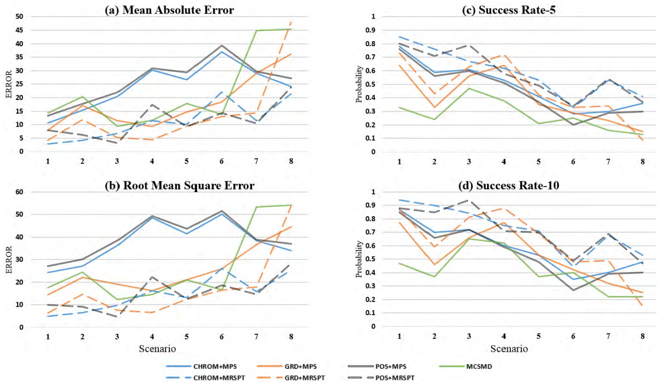
FIGURE 9. Table II-V are visualized as (a)-(d) for easier comparison and discussion. The number in the x-axis represents the order of Scenario. The dotted lines are the results of MRSPT with different iPPG recovery algorithms. In view of every metric, the best algorithms in each scenario are achieved integrating MRSPT.
