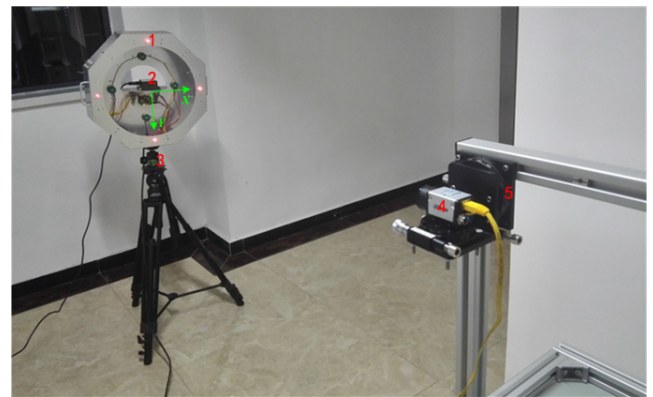
FIGURE 11. Experimental condition. (1) LED fixed on the disk target, (2) 2-axis inclinometer, (3) 3D rotation stage, (4) COMS camera, (5) 2D rotation stage for leveling.
