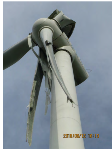
FIGURE 13. Three damaged blades.
