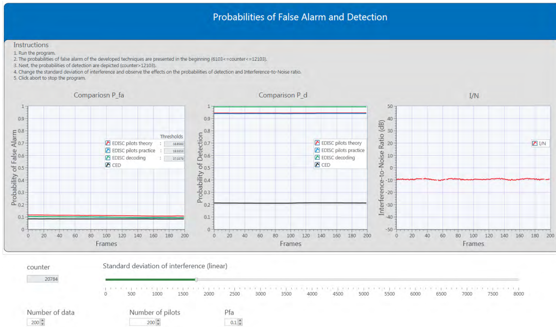
FIGURE 16. Visualization of the probability of detection of EDISC with pilots, EDISC with decoding errors and CED for INR \approx -10 dB.
