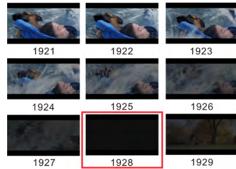
(a) A sub video with shot boundary, 1928th frame is fade out shot transition
