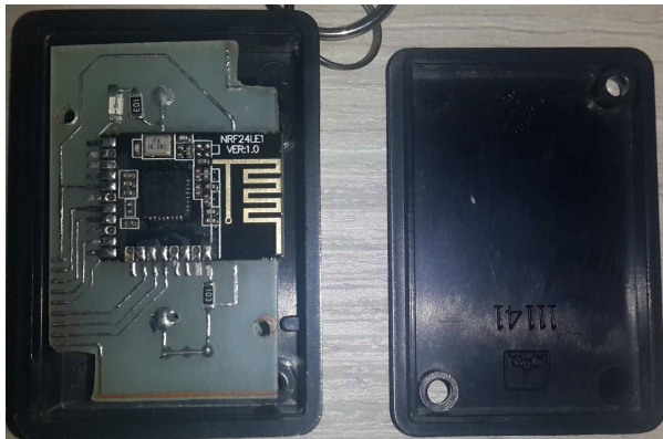
FIGURE 11. The implemented SmartTag prototype.
