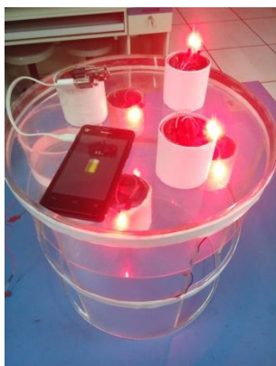
FIGURE 12. An application of the SR-TX-RXs WPT system charging multiple LEDs and mobile phones.
