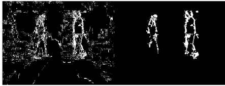
FIGURE 3. Detection of the moving object. Original image is acquired from the combination of the XORed bit planes and the thresholded image.
