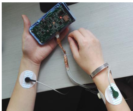
FIGURE 9. Self-developed single-lead ECG signal acquisition device.
