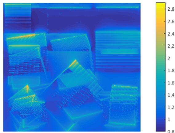
FIGURE 3. Cross section of peak electric field strength in MV/m, maximum value over x projected onto the y - z plane.
