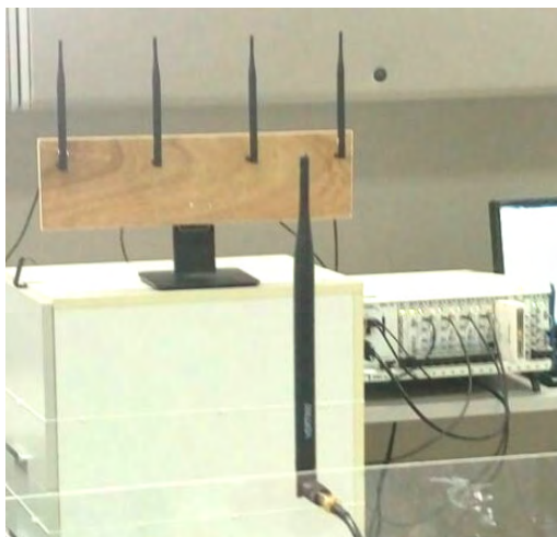
FIGURE 1. A uniform linear array (ULA) and a single source in the far-field region of the ULA.
