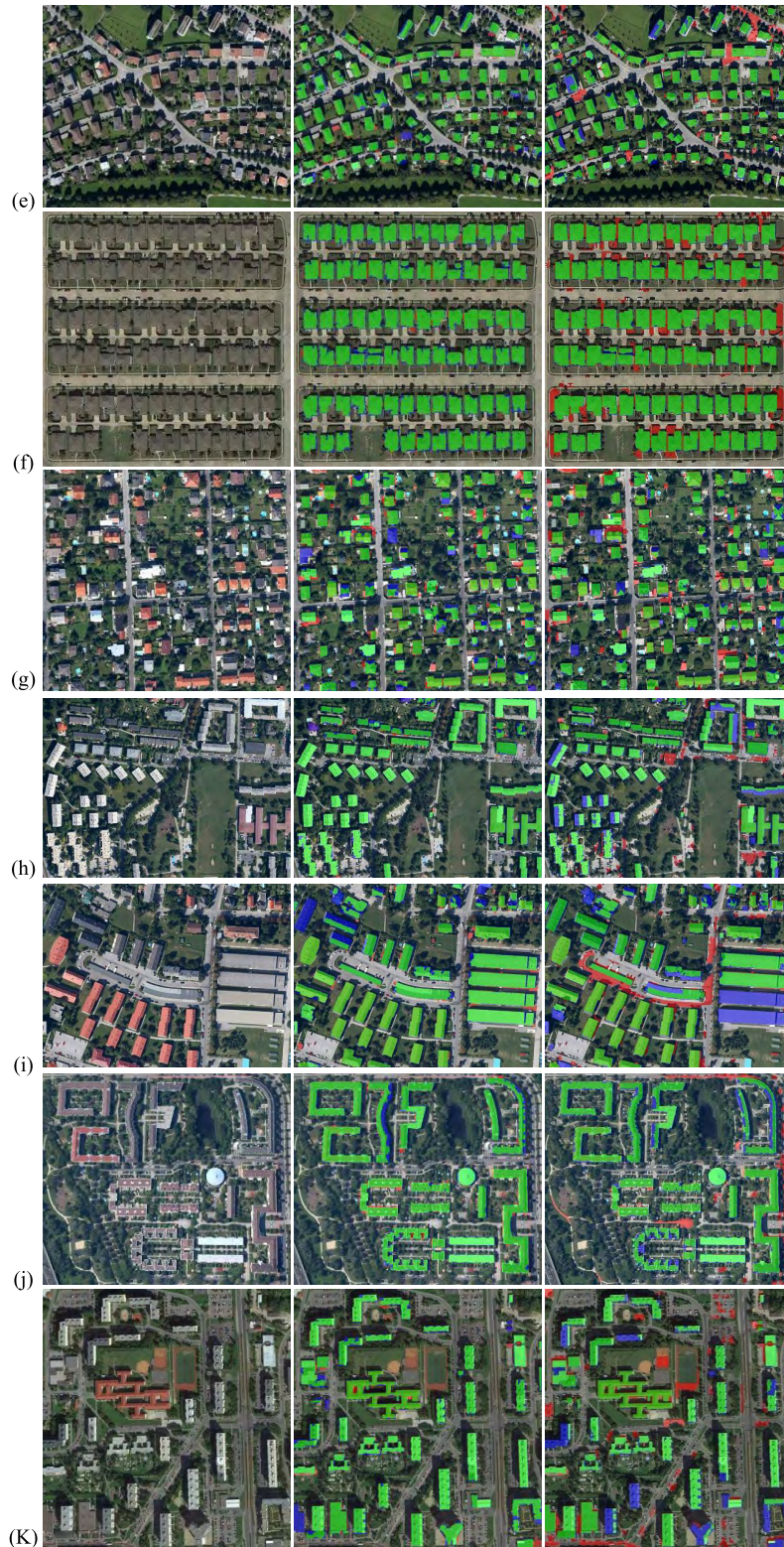
FIGURE 7. (First column) Test patches (e)–(k). (Second column) The results of the proposed method. (Third column) The results of the SD-PAC (Ghaffarian [34]) where the colours green, red and blue represent TP, FP and FN pixels, respectively.
