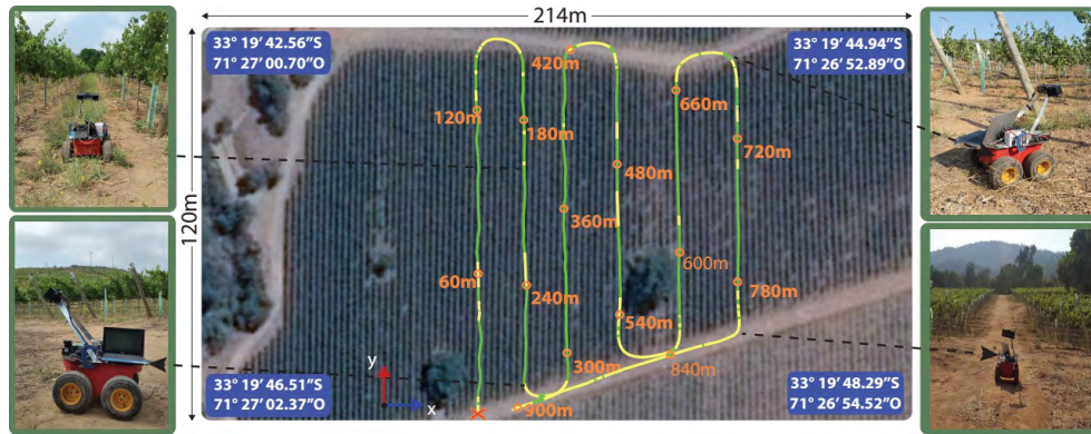
FIGURE 8. Long range test environment. The center of the picture shows a satelital image of the agricultural environment where the experiments were carried out –Vineyard of Casa Blanca, Chile. The side images show snapshots of the vehicle in-situ when traversed the pointed places. The trajectory of approximately 900m-long traversed two types of surfaces: grass and plowed terrain, as shown respectively in the green and yellow solid lines of the reconstruction of the travelled trajectory by the robot within a Cartesian coordinate reference system.
