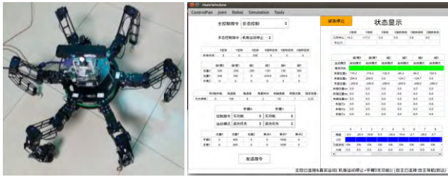
FIGURE 18. Wheel-leg compound mobile robot and its software console interface.
