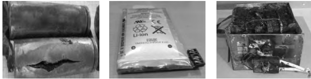
FIGURE 19. Safety problems of lithium-ion batteries.
