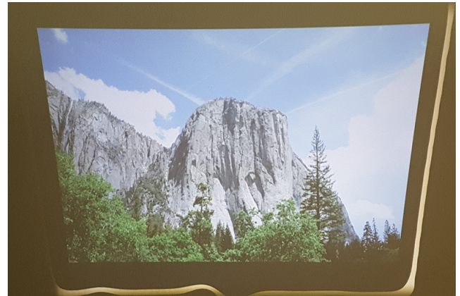
FIGURE 14. Keystone distortion caused by tilting the projector 20 degrees upward from the ground.
