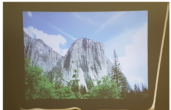
FIGURE 15. Keystone correction in the horizontal direction in the distortion shown in Fig. 14.
