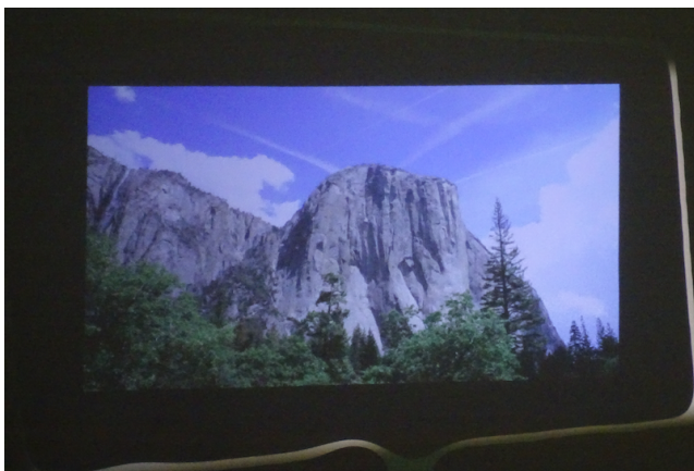
FIGURE 18. Keystone correction in the horizontal and vertical direction in the distortion of Fig. 17.
