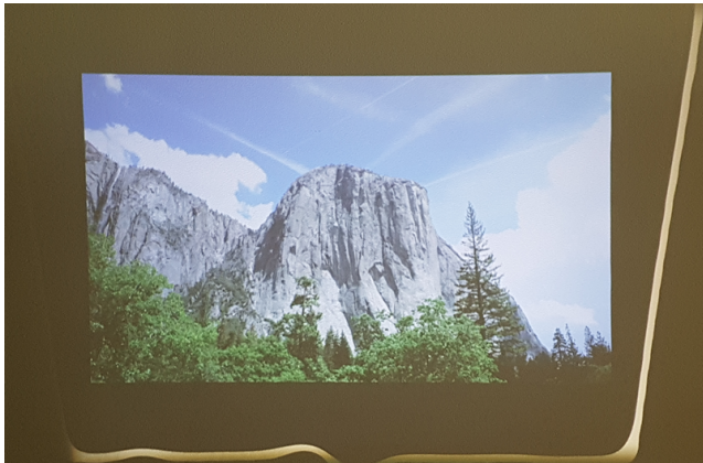
FIGURE 16. Keystone correction in the horizontal and vertical directions in the distortion shown in Fig. 14.
