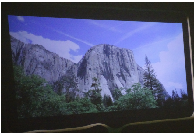
FIGURE 17. Keystone distortion caused by tilting the projector 15 degrees to the left.
