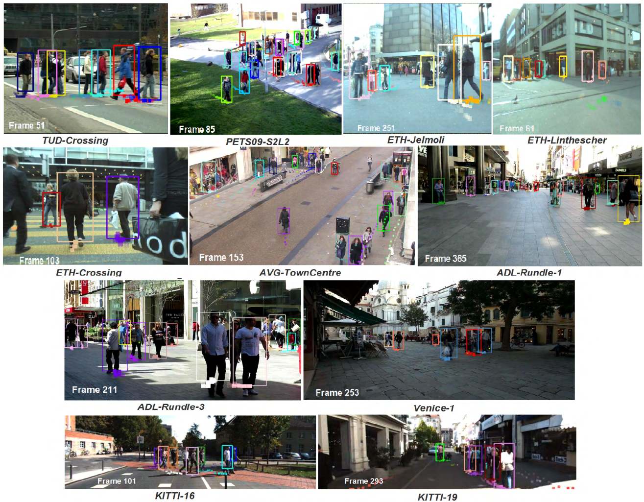
FIGURE 4. Qualitative performance of our proposed method on the test video sequences of the 2D MOTChallenge 2015. Different colors of the bounding boxes and trajectories demonstrate the identities of tracked targets.
