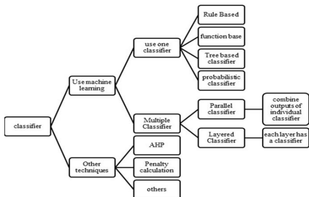
FIGURE 5. Classification of detection method.
