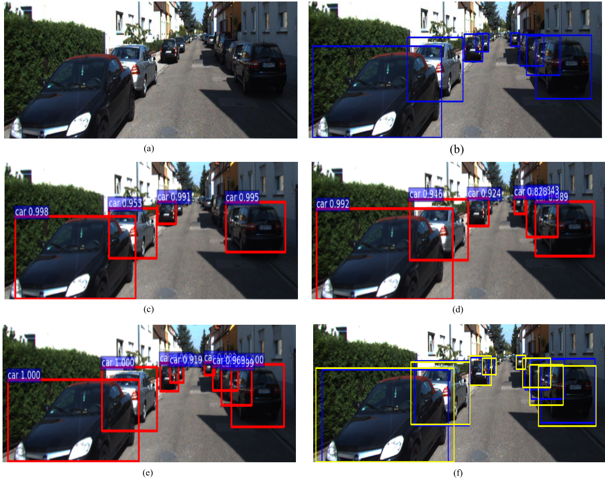
FIGURE 6. Comparison of small object detection. (a) Original image; (b) Ground truth; (c) Faster R-CNN; (d) Fusion of RPN and MCFF; (e) Proposed algorithm; (f) Comparison between (e) and (b).
