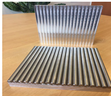
FIGURE 14. Aluminium mould employed for the bending of the row-by-row unit cell FSS.
