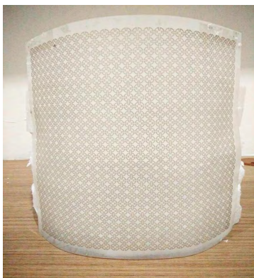
FIGURE 12. Experiment set-up used to evaluate the performance of the finite FSS array.
