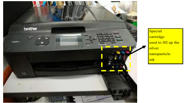
FIGURE 9. Brother MFC-J430W printer with special cartridge filled with silver nanoparticles ink used for fabricate the FSS prototype.
