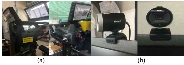
FIGURE 7. (a) FLIR S65 thermal camera, (b) visual camera.
