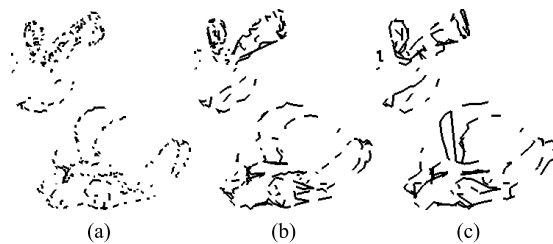
FIGURE 4. The parameter r controls the connected ridge-valley lines length. The larger the value of r , the length the connected the ridge or valley segment lines. (a) r=0.1 . (b) r=0.2 . (c) r=0.3 .
