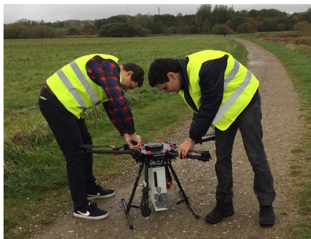
FIGURE 1. Preparation for UAV channel measurement: Our pilot is mounting the R&S scanner on the DJI Matrice 600 drone.
