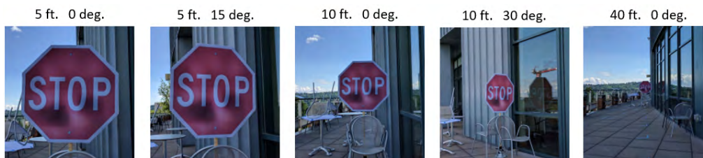
FIGURE 7. Example of road sign attack [75]: The success rate of fooling LISA-CNN [75] classifier on all the shown images is 100%. The distance and angle to the camera are also shown. The classifier is trained using LISA dataset for road signs [174].
