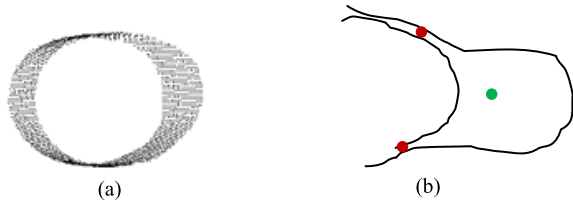
FIGURE 6. Middle points of 2D strap-like cross section point sets with non-uniform width.
