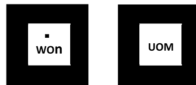
FIGURE 8. Example of two similar markers having a 0.64533 degree of similarity with each other (as calculated in FMO). If one of these markers already exists in the library, the FMO will not allow user to add the second one.
