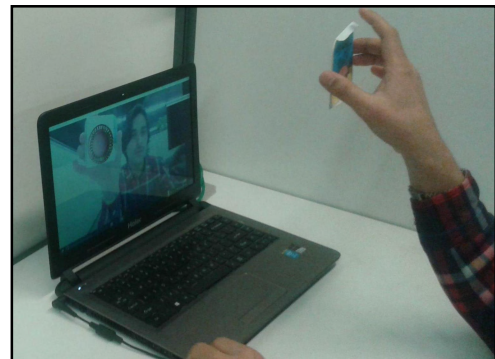
FIGURE 10. Experimental setup. The marker is in a continuous movement in front of the camera and the results (i.e., number of identifications and CF values) are continuously being stored in a text file.
