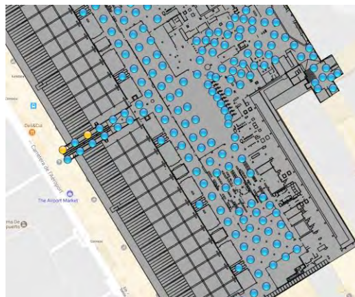
FIGURE 4. Fingerprinting Grid (PMI airport, Floor 4).
