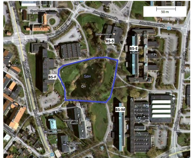
FIGURE 1. Aerial photo of the measurement area. Base station locations are indicated by labels BS-E (Latitude: 55.711131, Longitude: 13.210225), BS-S, BS-F and BS-M. The measurement route is plotted in blue color.
