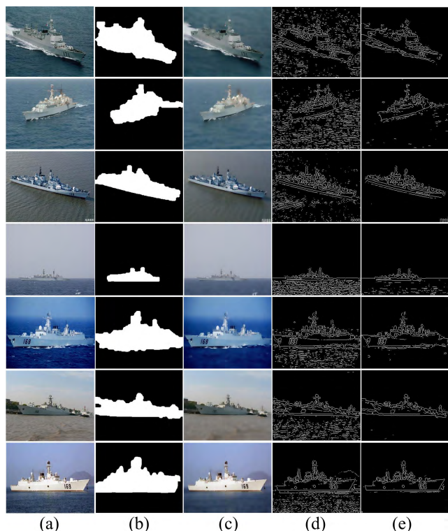
FIGURE 7. Visual image smoothing results. (a) The original visual images; (b) The target detection results; (c) The smoothed visual images; (d) The edge maps of the original visual images; (e) The edge maps of the smoothed images.
