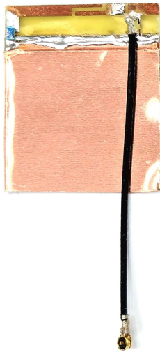
FIGURE 2. Photo of the prototype made of a 0.4-mm-thick FR4 substrate and fed by a 50-Ω mini-coaxial cable of length 40 mm.
