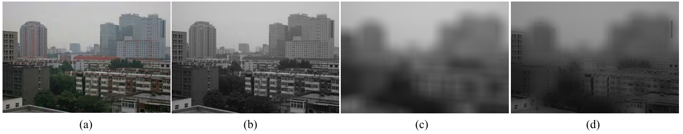
FIGURE 3. Estimation of transmission map. (a) Hazy image. (b) Minimum filtering. (c) Average filtering. (d) Grayscale optimization.
