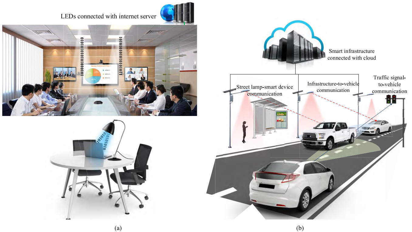
FIGURE 7. Selected application scenarios of VLC/LiFi systems, (a) indoor environment, (b) outdoor environment.
