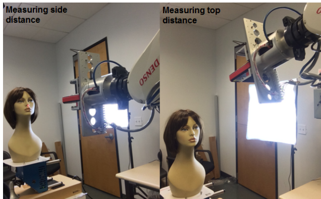
FIGURE 6. Using laser meter on robotic arm to measure the side and top distance.
