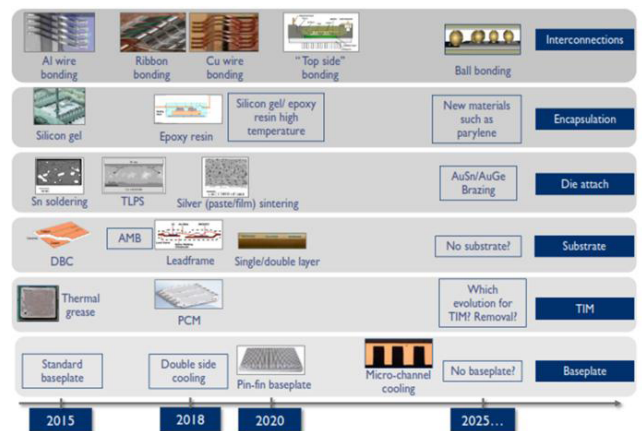
FIGURE 7. The development of packaging technology for IGBT modules [9].
