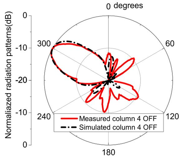
**FIGURE 16.** Simulated and measured radiation patterns of single-beam mode when column 4 OFF at 5.2 GHz in azimuth plane.
