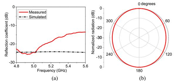
FIGURE 5. Simulation results of the monopole antenna: (a) Reflection coefficient. (b) Normalized radiation pattern at 5.2 GHz.
