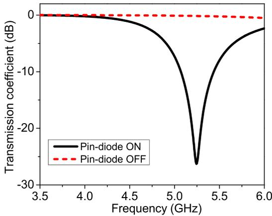
FIGURE 2. Simulated transmission coefficients of FSS unit-cell in different pin-diode states.
