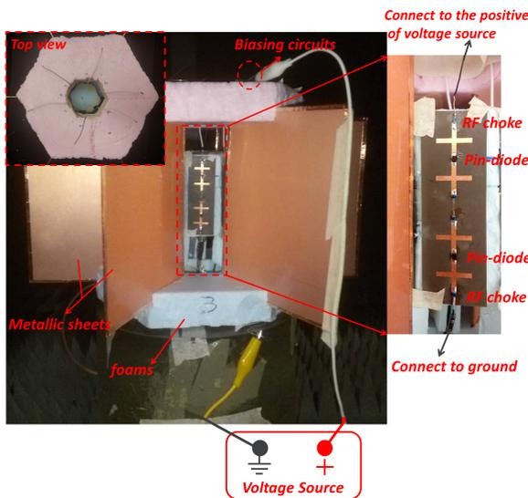
FIGURE 13. Photograph of the fabricated antenna in anechoic chamber.
