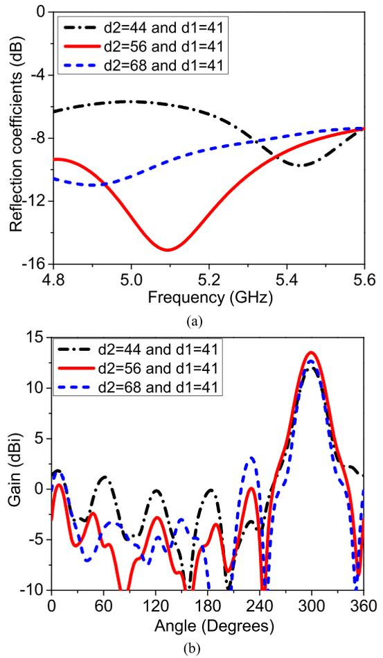
FIGURE 9. The effect of  $d2$  on the proposed antenna performances: (a) Reflection coefficients. (b) Gain.
