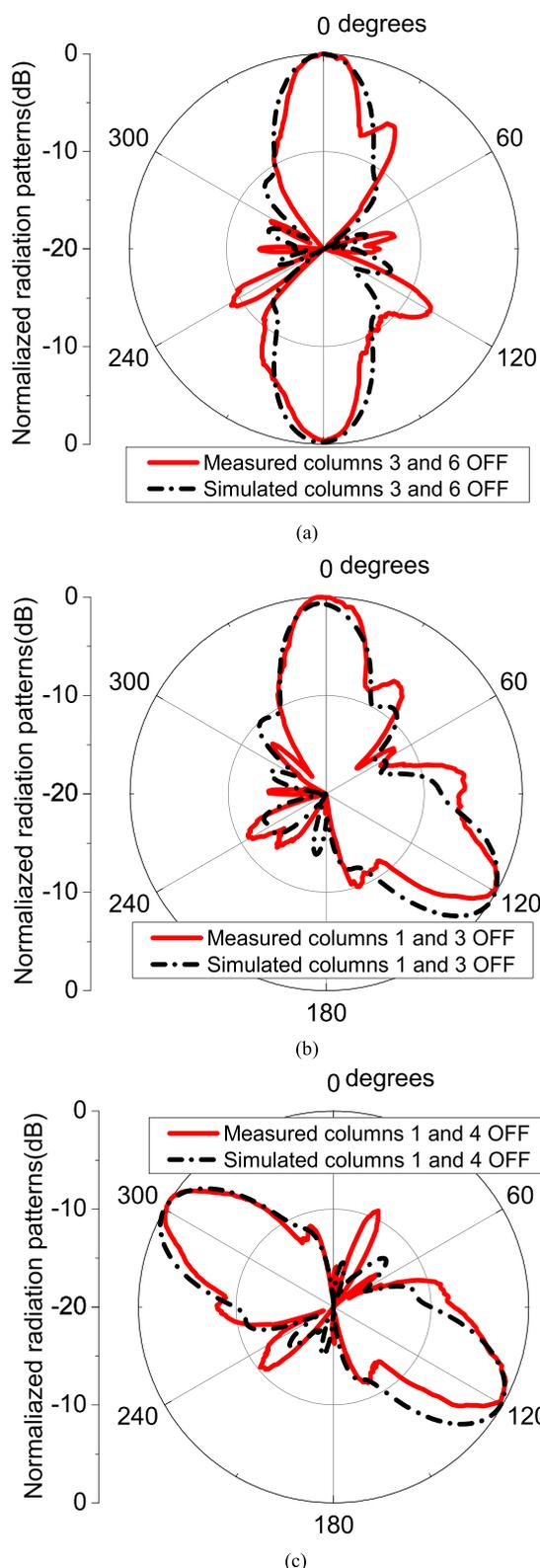
**FIGURE 17.** Simulated and measured radiation patterns of two-beam mode at 5.2 GHz in azimuth plane: (a) Columns 3 and 6 OFF. (b) Columns 1 and 3 OFF. (c) Columns 1 and 4 OFF.
