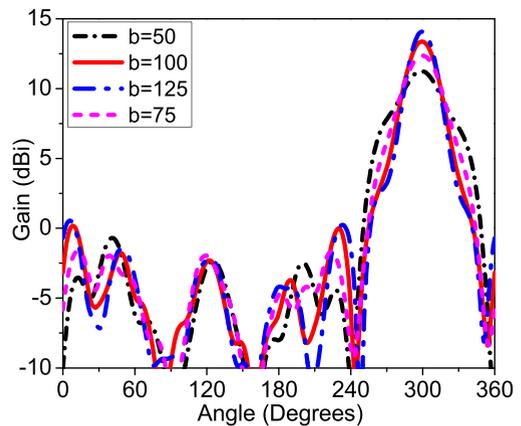
FIGURE 10. The effect of  $b$  on the radiation patterns of proposed antenna.
