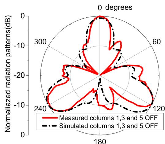
**FIGURE 18.** Simulated and measured radiation patterns of three-beam mode at 5.2 GHz in azimuth plane when column 1, 3 and 5 OFF.
