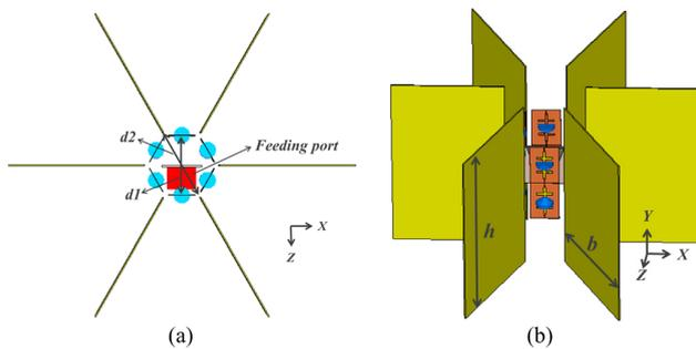
FIGURE 3. Proposed beam-switching with high gain antenna structure: (a) Top view, (b) Side view.
