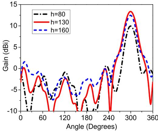
FIGURE 11. The effect of  $h$  on the radiation patterns of proposed antenna.
