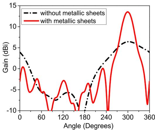
FIGURE 12. Simulated radiation patterns of antenna with and without metallic sheets in the azimuth plane at 5.2 GHz.
