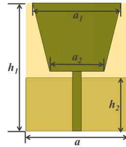
FIGURE 4. Structure of the monopole antenna.
