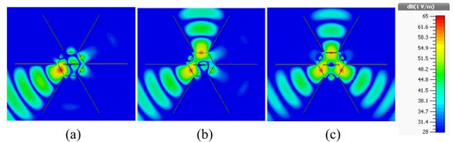
FIGURE 7. E-field distribution of the antenna at 5.2 GHz: (a) Single-beam mode. (b) Two-beam mode. (c) Three-beam mode.
