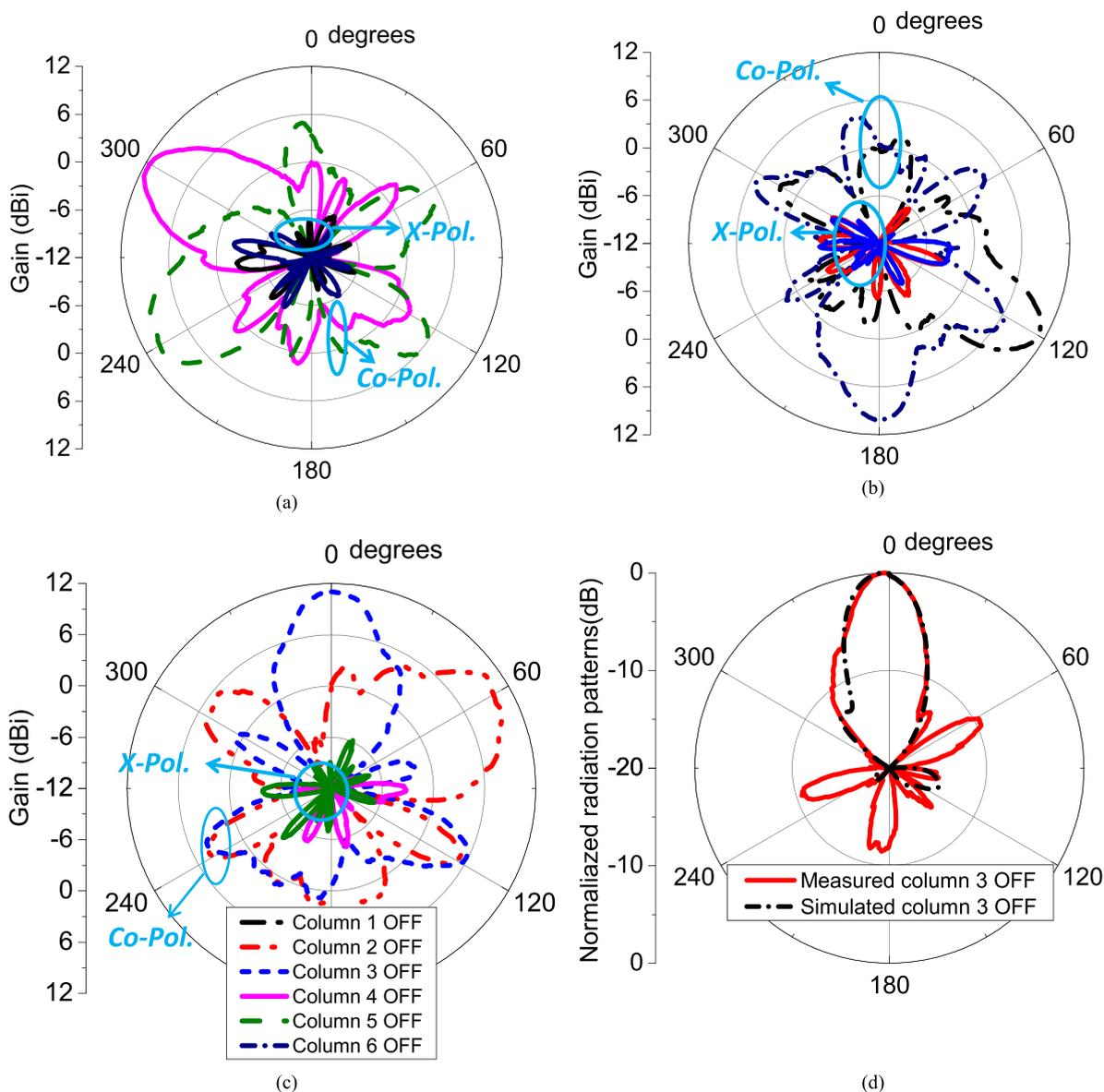
FIGURE 15. Measured radiation patterns of a single-beam mode at 5.2 GHz: (a), (b) and (c) in azimuth plane, (d) in elevation plane.
