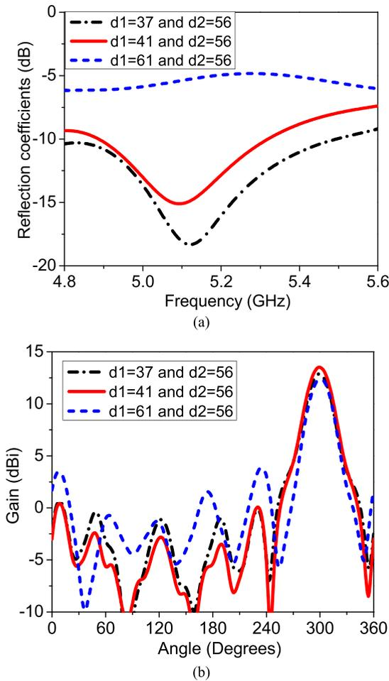
FIGURE 8. The effect of  $d1$  on the proposed antenna performances: (a) Reflection coefficients. (b) Gain.
