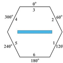
FIGURE 6. Schematic diagram of beam-switching antenna.
