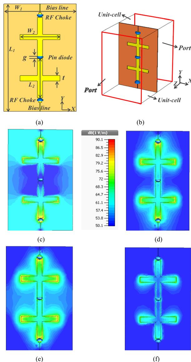
**FIGURE 1.** (a) Geometry of FSS unit-cell. (b) Configuration of FSS unit-cell simulation. (c) E-field distribution at 2.5 GHz. (d) E-field distribution at 4.8 GHz. (e) E-field distribution at 5.2 GHz. (f) E-field distribution at 5.8 GHz.
