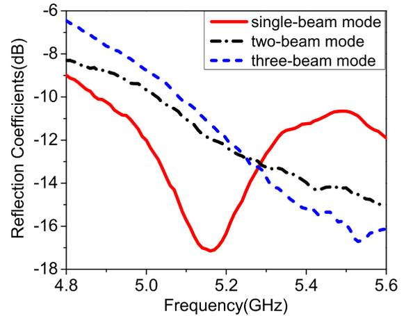
FIGURE 14. Measured reflection coefficient results of proposed antenna in different modes.
