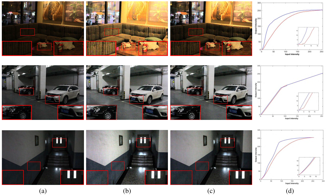
FIGURE 4. Contrast enhancement results in Restaurant , Car , and Classroom by HE, OCTM [6] and AGCWD [7]. (a) Original image. (b) Enhancement by the original histogram. (c) Enhancement by the noise aware histogram. (d) Mapping curve by the original histogram (blue) and the noise aware histogram (red). The first row is processed by HE, the second one by OCTM and the third one by AGCWD. The enhanced color images are obtained by Section III-C.
